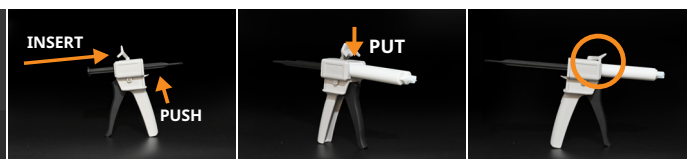
① Push the latch and insert the stick. ② Put the tube in. ③ Close the cover.
